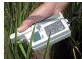
葉色測定 Measurement of leaf color
